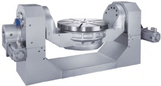
Rotary Axis - DDM (80rpm, option 800rpm) Tilting Axis - Tandem drive by spur gear and worm gear
